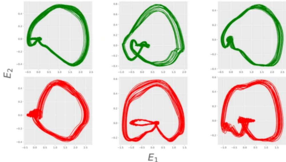
Two dimensional projections of embedded attractors for ECG signals for three healthy (top panel) and three unhealthy (bottom panel) cases. All the attractors are plotted using the SVD transformation.
